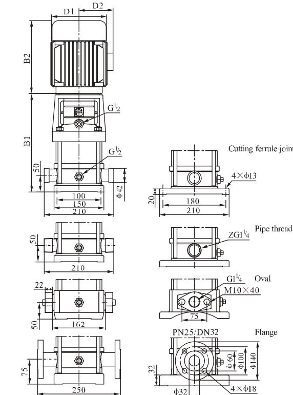
CDL4-19~4-22 sub-connection of pipeline has no oval flange connection.
