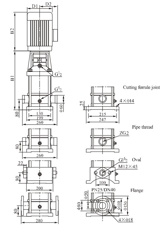
CDL8-14~8-20 sub-connection of pipeline has no oval flange connection.
