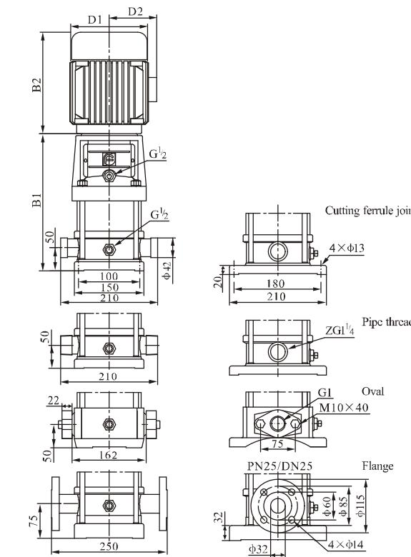
CDL2-18~2-26 sub-connection of pipeline has no oval flange connection.
